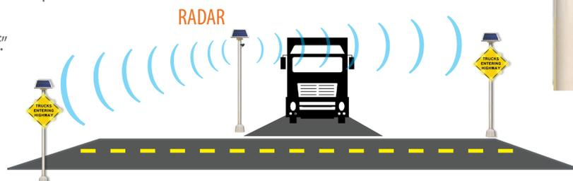
The **Radar** detects a vehicle and triggers the **Sign Alerts** to flash for a set amount of time to warn drivers of vehicles entering the highway.
