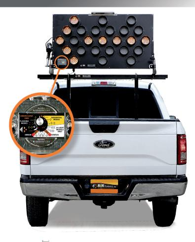
• low profile mount with auto raise/lower • 12V linear actuator • over-the-cab mounting hardware
