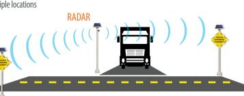
The **Radar** detects a vehicle and triggers the **Sign Alerts** to flash for a set amount of time to warn drivers of vehicles entering the highway.
