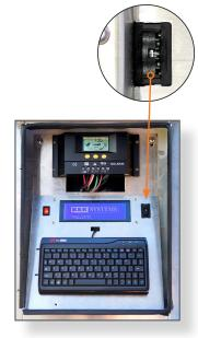
**K&K Systems' Quick Message Selection** Thumbwheel switches between the first 16 user defined messages. Roll the thumbwheel to desired message number to display a message.
