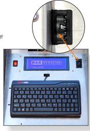
**K&K Systems' Quick Message Selection** Thumbwheel switches between the first 16 user defined messages. Roll the thumbwheel to desired message number to display a message.
