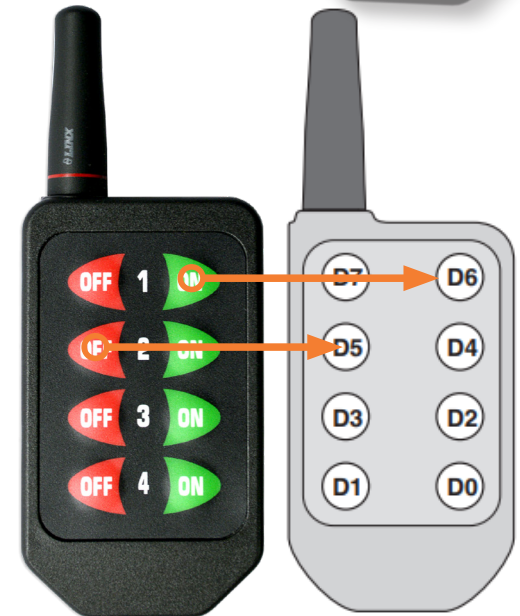
Key Fob buttons as they are related to the internal DIP Switches.
